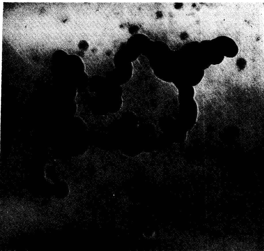
FIG. 1. A. Transmission electron micrograph of a carbon filament showing the internal structure of the more transparent areas ( \times 49,500 ). B. Transmission electron micrograph of an exceptional filament which has formed by spiral growth ( \times 23,250 ).
